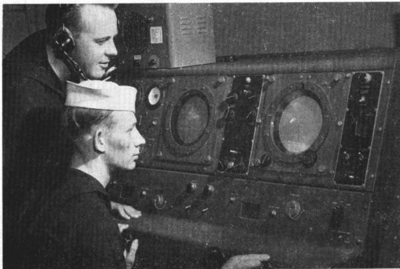
HUNTING-Radarmen practice searching for pips. Analysis and location of contacts by RDs may some day determine the safety of their ship.
